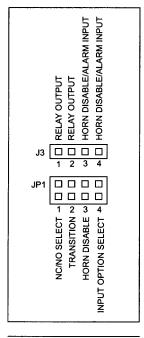
Figure 2: Configuration/set-up options
