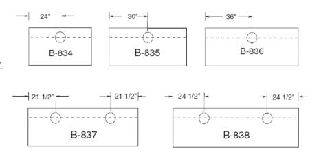
Duct collar locations are as shown above. The center line of each collar is 8" from the back of the hood. The area indicated by the dashed lines is designated for plumbing and electrical rough-ins. All rough-ins should be kept within 7" of the wall and 18" from the floor.
