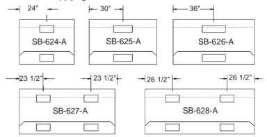
Duct collar locations are as shown above. The center line of each collar is 8" from the back of the hood. The center line of the supply duct is 35 5/8" from the back of the hood. The area indicated by the dashed lines is designated for plumbing and electrical rough-ins. All rough-ins should be kept within 7" of the wall and 18" from the floor.
