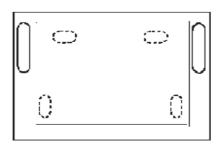
Fume Hood work surfaces are molded from a modified epoxy resin that has been especially compounded and cured to provide optimum physical and chemical resistance required for a heavy duty laboratory working surface. Countertops are 1" thick with a 3/8" deep dishing to contain spills and have a non-glaring black finish.
