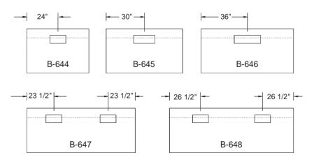
Duct collar locations are as shown above. The center line of each collar is 8" from the back of the hood. The area indicated by the dashed lines is designated for plumbing and electrical rough-ins. All rough-ins should be kept within 7" of the wall and 18" from the floor.
