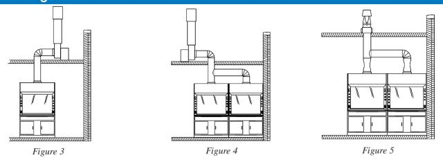
Whenever possible exhaust blowers should be located on the roof of the building. This will insure that the ductwork inside the building will remain under negative pressure preventing leakage of contaminated air into occupied spaces.
