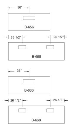
Duct collar locations are as shown above. The center line of each collar is 8" from the back of the hood.
